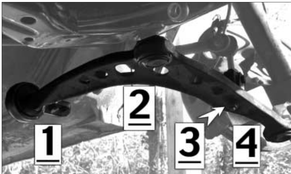
1. CONTROL ARM BUSHING IN BRACKET 2. INNER BALL JOINT 3. SWAY-BAR LINK AND NUT 4. OUTER BALL-JOINT
